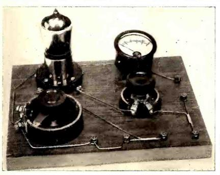
Photograph of the completed vacuum tube voltmeter described by the author
